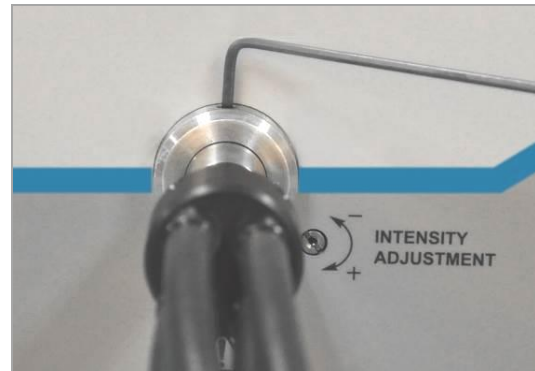
Figure 2. Gently Tighten Setscrew on Lightguide Mount with Hex Wrench
