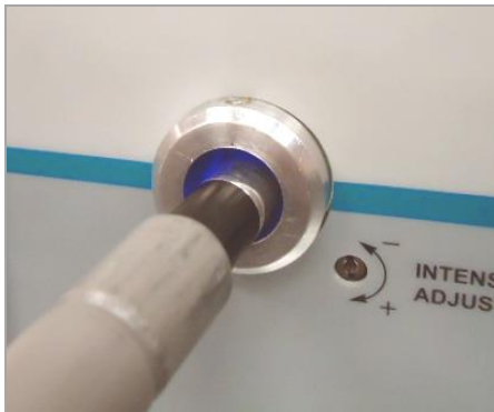
Figure 1. Insert Lightguide into Lightguide Mount
