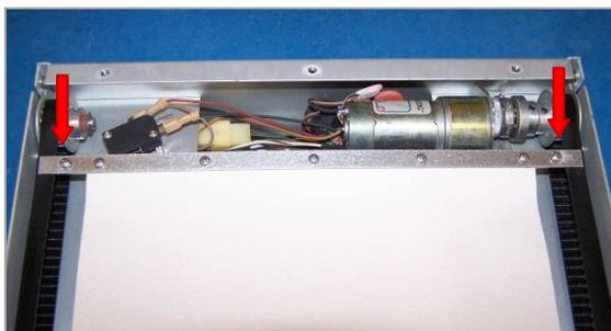
Figure 5. Loosen End Screws
