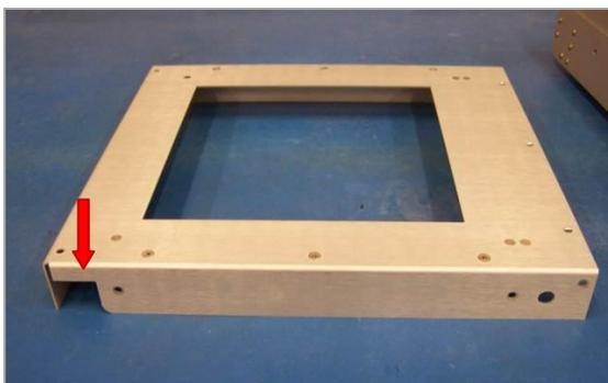
**Figure 12.** Roller End of the Bottom Housing Plate
