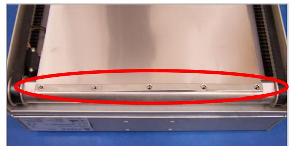
Figure 6. Five 2-mm Retaining Screws
