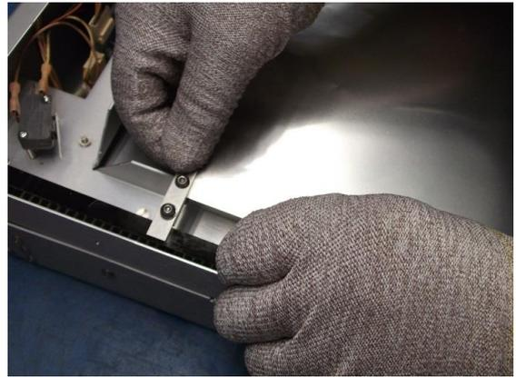
**Figure 8.** Slide the Clamp Bar onto the Belt
