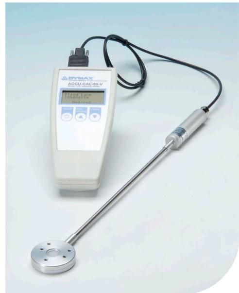
ACCU-CAL™ 50V for measuring floods and conveyors only PN 40044
