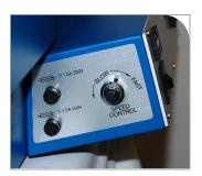
Conveyor belt speeds can be adjusted by turning the speed control knob, located on the side of the conveyor control panel. Belt speed is indicated on the speed display indicator. The belt speed knob is a ten-turn potentiometer and is equipped with a lock.
