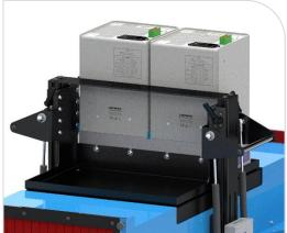
3. Place the remaining two systems side-by-side onto the conveyor cradle. Align the 4 spacer screws with the 4 slots. (Figure 13).
