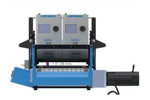
Cradle at minimum height Tunnel clearance is 1.5" (38 mm)
