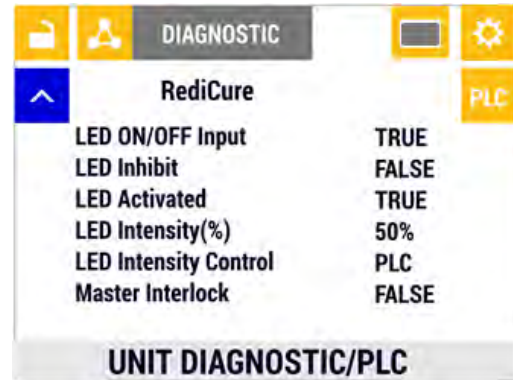
Figure 45. PLC Screen, UV LED Activated (On)
