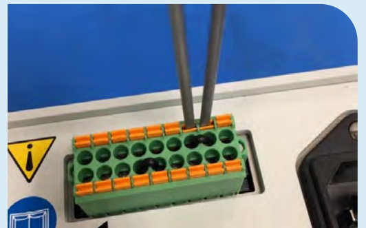
Figure 11. Remove Jumper from Terminal Block
