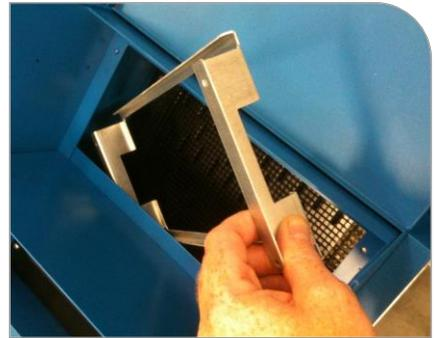
Figure 1. Installing Frames through Cradle Opening
