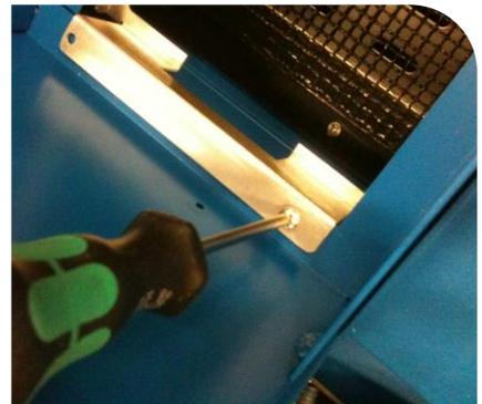
Figure 2. Installing Frame Tab
