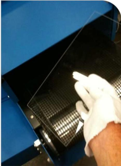
Figure 5. Installing Quartz Window in Conveyor
