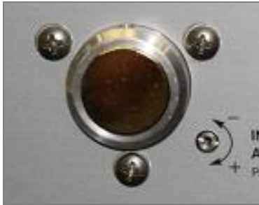
Figure 5. Shipping Cap in Lightguide Mount
