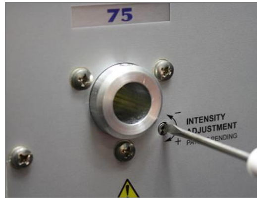
Figure 8. Adjusting Intensity with a Screwdriver
