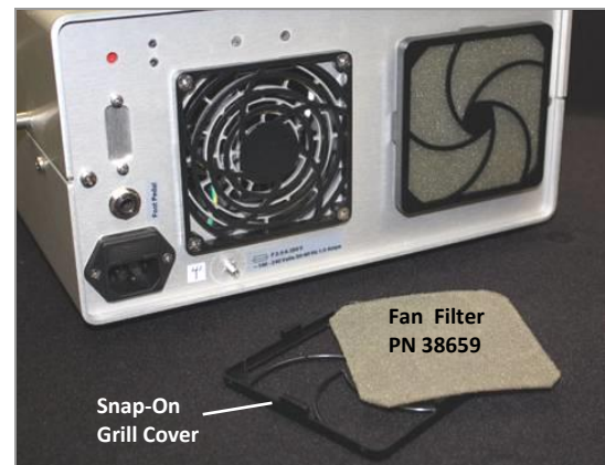
Figure 15. Fan Filter Replacement
