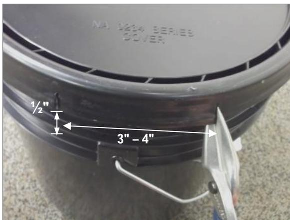
Figure 2. Place the Cutting Tool Under the Cover Skirt and Cut  $\frac{1}{2}$ " Slits from the Bottom Up, 3"-4" Apart
