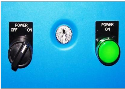
Figure 11. Main Power Controls
