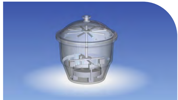
Figure 4. Representation of a Flowers of Sulfur Test Chamber
