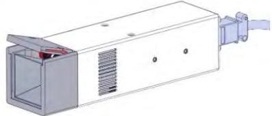
4. Slide the damaged glass cover out (Figure 6), taking care not to touch the metallic reflector surfaces.
