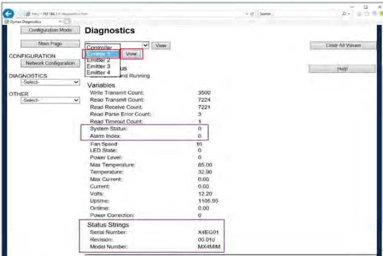
Expansion module hours are accumulated but will not reset when a BlueWave QX-4 head is replaced. It is suggested to monitor BlueWave QX-4 LED head hours separately for process control. The MX-4E is tracked as “Emitter” under Run Hours.
