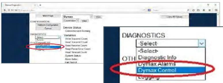
11. Verify that all connected emitters can be turned ON/OFF via ON/OFF selection. Selecting the appropriate radio button on/off, press the Update Emitters Button and observe the emitter illumination.
