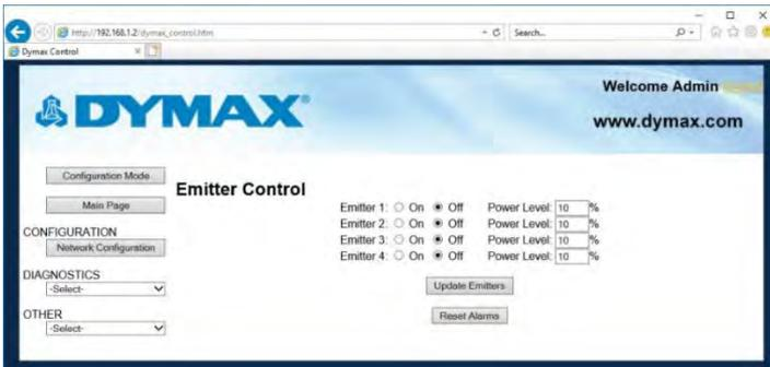
**NOTE:** This page is only available when the device is not being controlled by Ethernet protocol commands.
