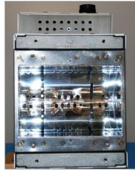
4. Mount the Irradiator(s) into the conveyor's Lamp Support (Figure 17 and Figure 18). Take particular care not to damage the protective Screen Covering the lamp end of the Irradiator.
