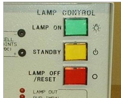
**NOTE:** The Fusion Power Supplies are interlocked with the Conveyor so that the Conveyor must be operating and the Conveyor Chain in motion before the Lamps will ignite.
