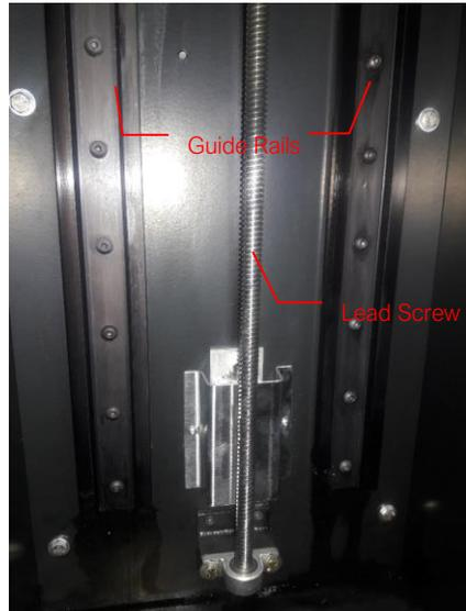
5. Once the lead screw and the two guide bars have been appropriately cleaned, the assemblies will need to be properly lubricated.
