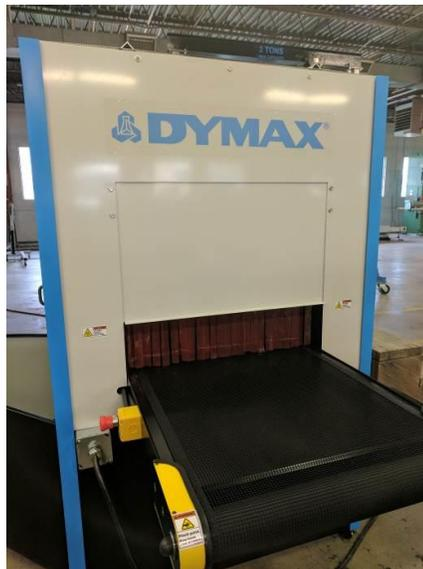
3. The irradiator is mounted on a linear stage that allows the height of the curing lamp to be adjusted from the conveyor belt. Use the control functions on the HMI to move the UV irradiator up or down as needed to allow for parts clearance and/or optimized cure height.
