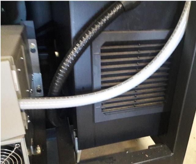
6. Once the fan cover has been removed, the fan filter can be lifted away from the assembly and replaced with a new filter.
