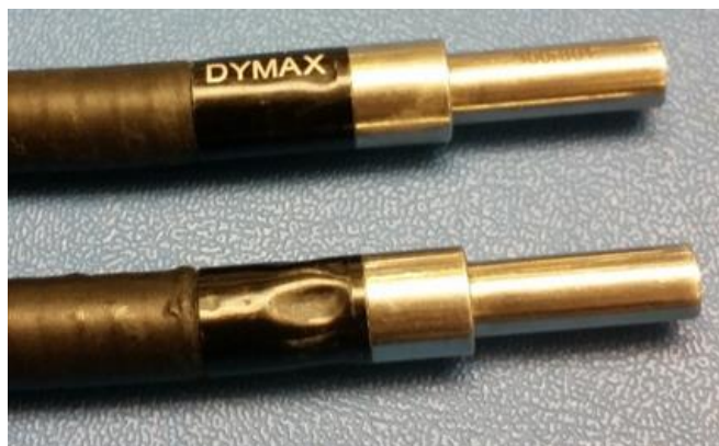
Figure 8. Damaged Lightguide Caused by Over Tightening
