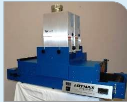
Figure 2. UVCS Conveyor System with Two Fusion Lamps
