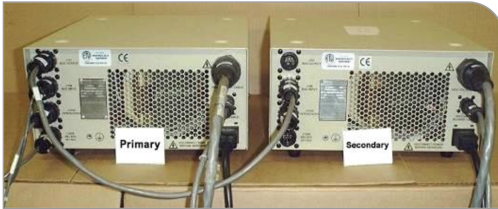
Figure 10. Power Supplies (Back)
