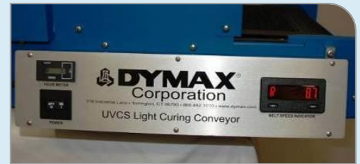
Figure 12. Conveyor Front Panel
