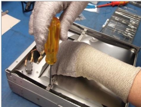
Figure 30. Tighten the M4 x 6 mm End Screws
