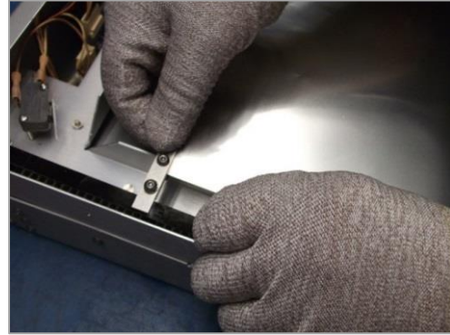
Figure 29. Slide the Clamp Bar onto the Belt
