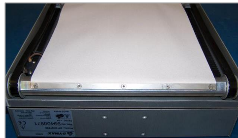
Figure 25. Inner Curtain Assembly (Kevlar Curtain Shown)
