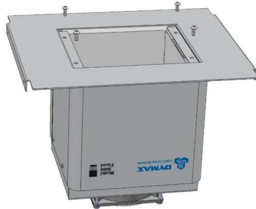
3. Install the assembly into the Manual Shutter and attach it with four 8-32 x  $\frac{3}{8}$ " screws. (Figure 5)
