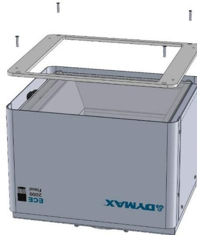
3. Install the two Mounting Plates (Figure 14) on the ECE 2000 Lamp Reflector Housing by installing the four M3 x 16 mm screws and four M3 flat washers.
