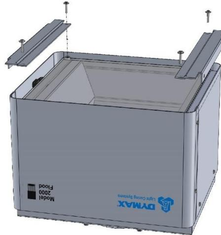
3. Install the assembly into the Manual Shutter and attach it with four 8-32 x 3/8" screws removed in instruction one (Figure 8).
