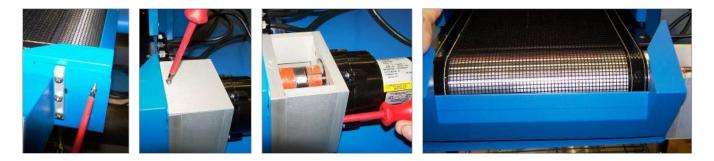
2. Remove all tension from the belt by turning the belt adjustment knobs counterclockwise as shown.
