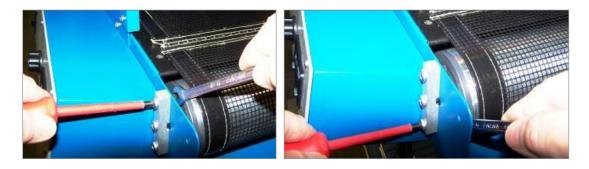
• Move the shaft assembly slightly to realign the drive roller and center the belt. Tighten the bolts when adjustment is complete.
