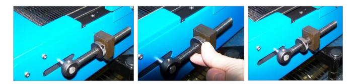
3. Manually move the belt splice to the end of the conveyor. Remove the fiberglass rod that ties the ends of the belt together. Remove the belt.
